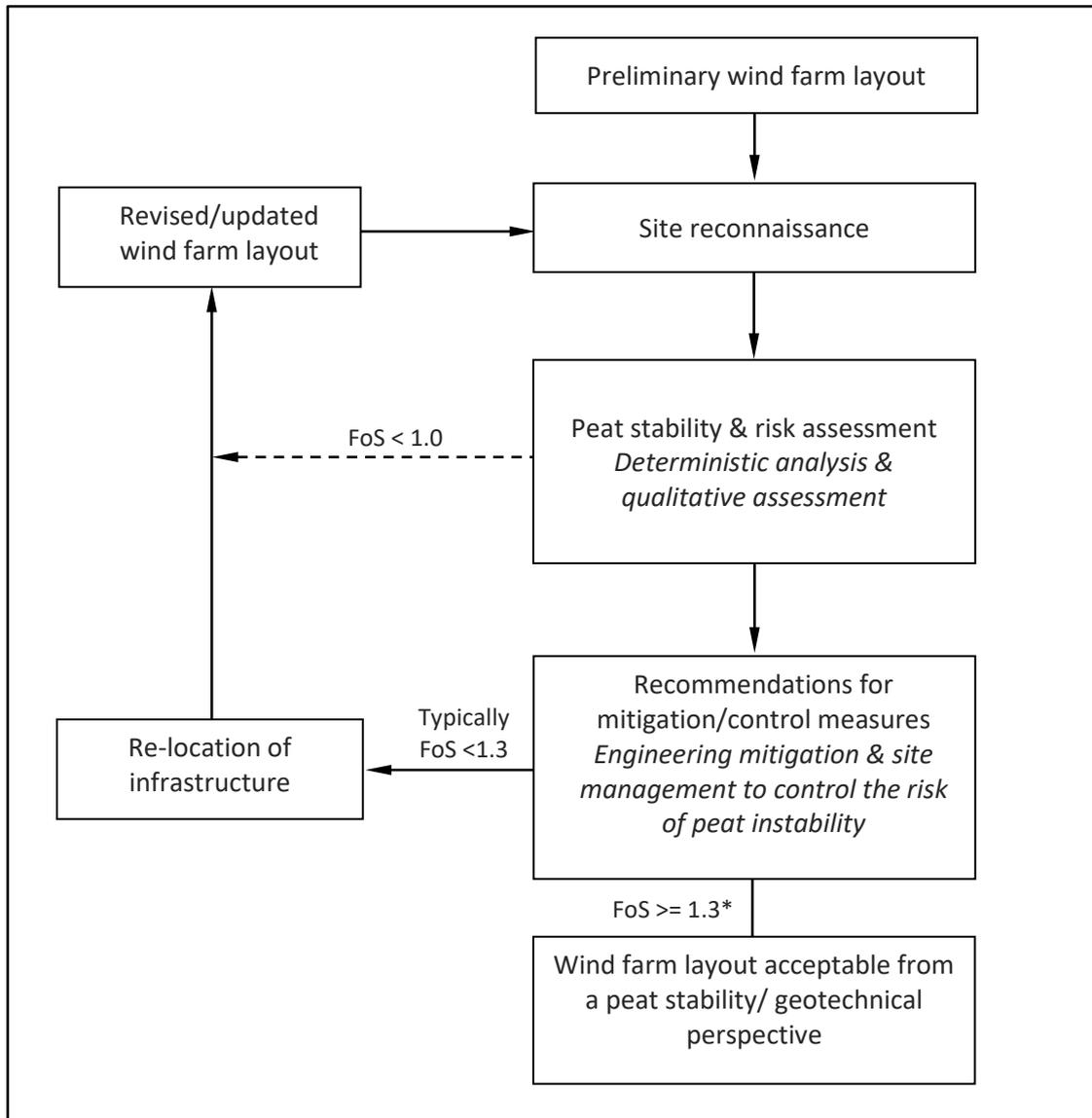
\*An FoS of between 1.0 and 1.3 does not mean that a failure will occur, but that the area requires attention. Mitigation measures can be provided for areas with an FoS of between 1.0 and 1.3 to reduce the risk of failure.
