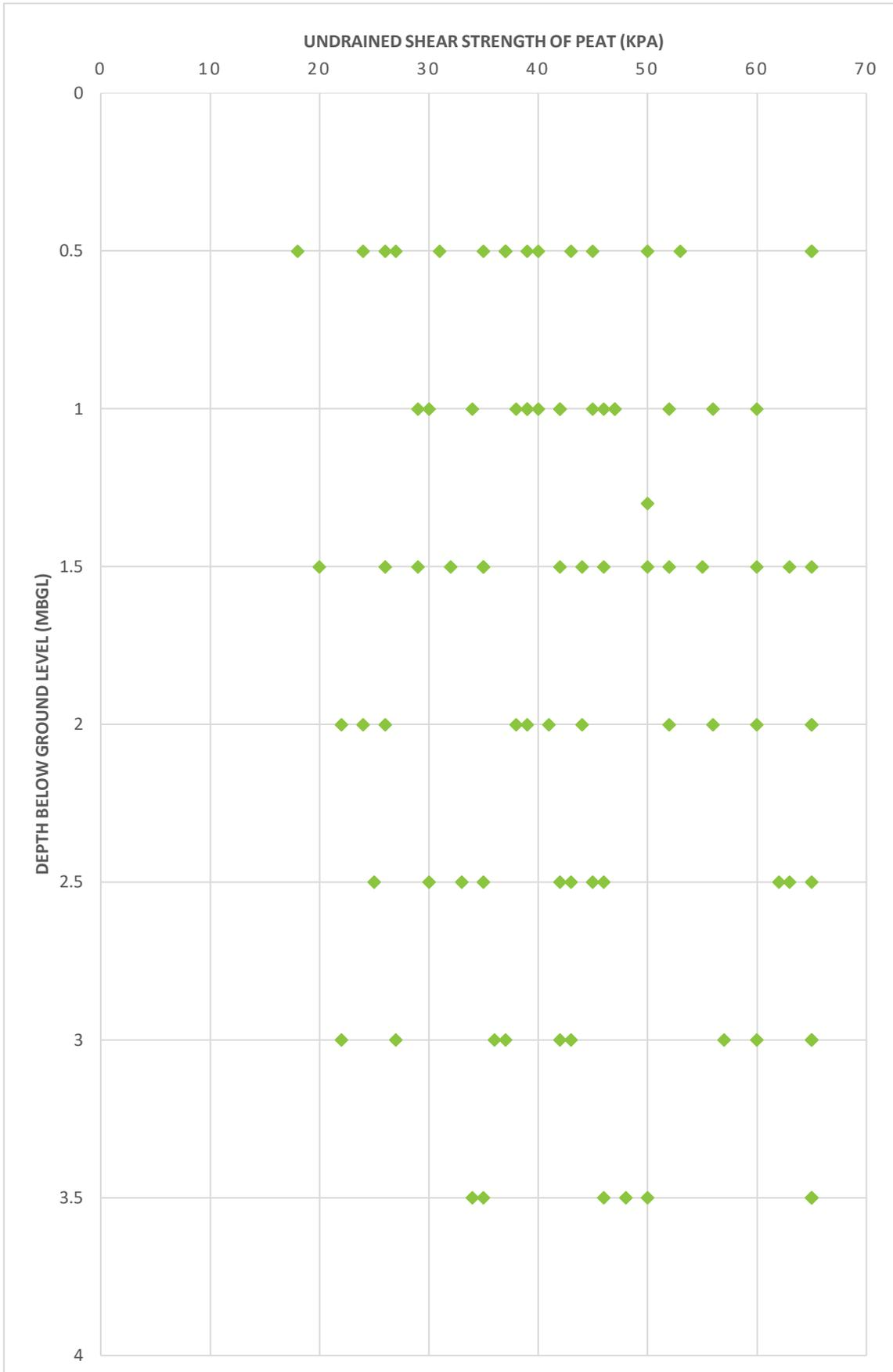
**Figure 5-1: Undrained Shear Strength ( $c_u$ ) Profile for Peat with Depth**
